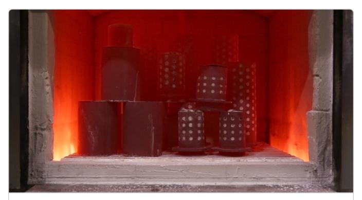
Place the casting flask in a cold furnace and heat according to the burnout schedule provided on page 2. Remove the mold from the furnace and cast metal.
