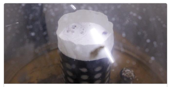
Degas the filled casting flask in the vacuum chamber for an additional 90 seconds or according to the manufacturer's instructions. Carefully remove the flask from the investment chamber and allow it to set in a vibration-free environment.
