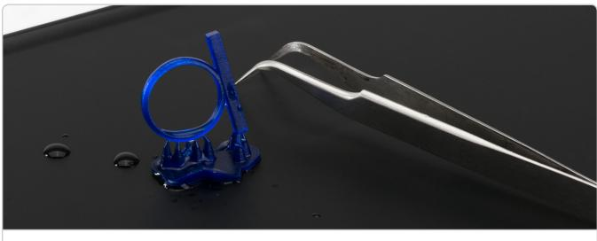
Allow the part to fully dry after removing it from the IPA bath.
