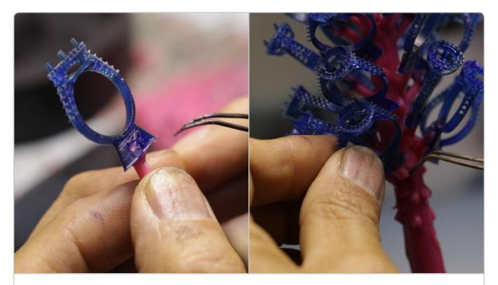
Add wax sprues and gates to the print as you would for lost-wax casting. Ideal positioning will vary with part geometry.
