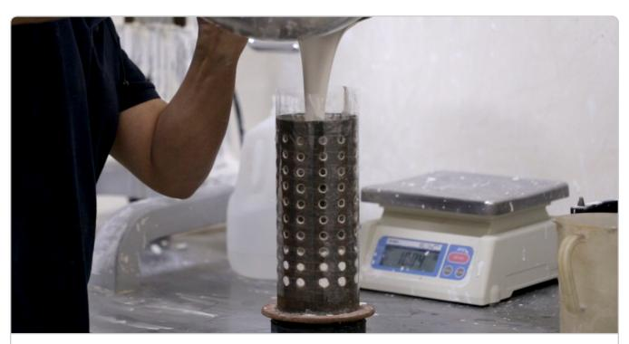
Slowly pour the investment into the casting flask. Pour the investment down the side of the flask to avoid damaging the fragile wax tree.
