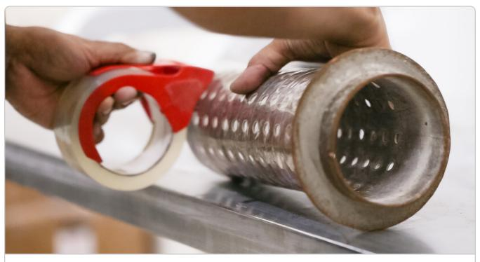
Attach a casting flask to the sprue base. If the flask is perforated, wrap it with clear packing tape to contain the investment.
