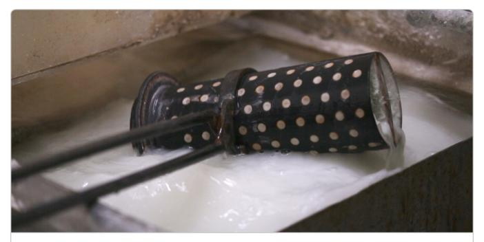
After casting, carefully quench the mold and wash away the investment.
