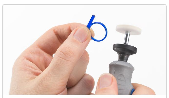
Polish the surface using polishing paper or a rotary tool with a buffing attachment.
