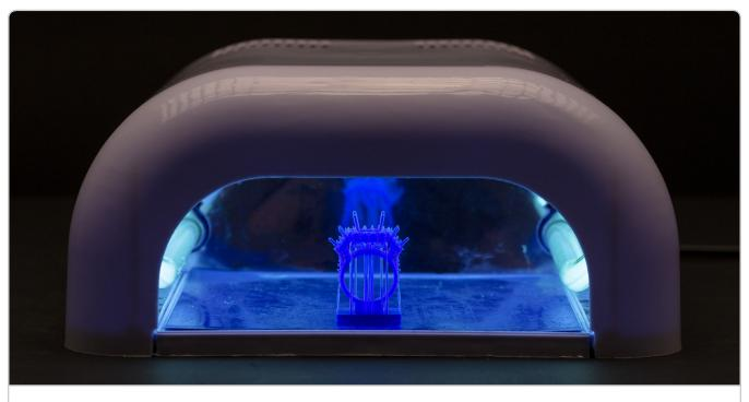
Cure the part under UV light until the surface is hard and rigid. Discoloration of the part is normal during this process.
