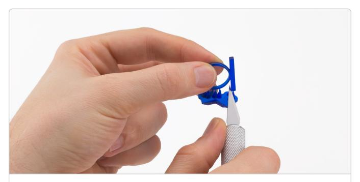
If necessary, carefully remove support material from your print. Using fine sandpaper (400 grit and above), gently sand away support marks.
